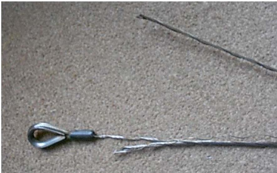
Further information from Simon is that, although he had inspected *Cynthia's* shrouds just over a month before this incident, closer inspection of the broken wires revealed rust on some of the ends, indicating that these had been broken for some time. These were missed during inspection or were not visible, but either way, they were certainly not obvious. As rigging failures are, fortunately, quite rare, Simon feels this
